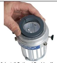
3. Install Optional Bushing if necessary. Line up slot openings. \*See Flexbar catalog or website for listing of available bushing adapters
