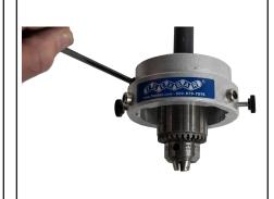
4. Install Clamp Assembly on Quill TIGHTEN CLAMP SCREW
