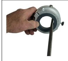
In the event that installing clamp on quill was too tight, it is possible to dress bushing material to fit.
