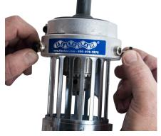
Make sure to tighten two cage locking thumb screws before operation. To remove cage, back out thumb screws, pull cage out of clamp body.
