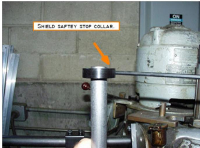
Next install the safety height stop collar at the top of the slotted pipe. At this time mate the X and Y axis pipes into their clamp body holes about halfway. (See image below)
