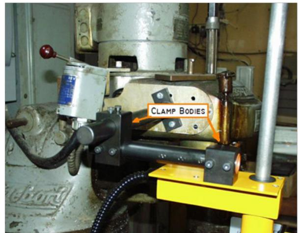
Slide the clamp bodies over the bars and tighten the hex clamping screws. You will need to readjust the X, Y and Z adjustments to position the shield properly. The trick here is to leave one of the two clamp screws loose while you position. After final position is established, tighten all screws in the clamp bodies.
